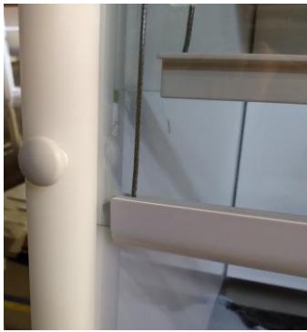
Figure 5. The lift limiter on the Fume cupboard.
