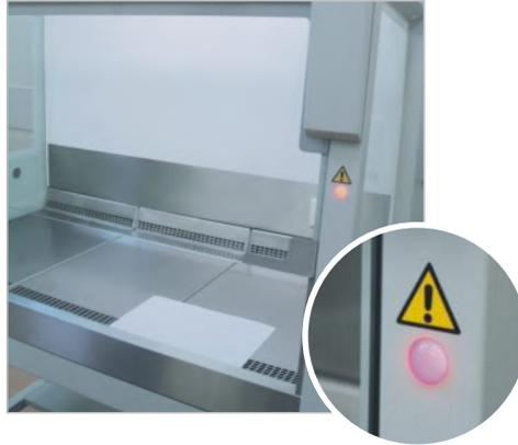
**Test:** Cover the front grille on the table top with a sheet of paper. The audible-visible indication system will work in 5 seconds. The display will show: **"BLOCKED CABINET AIR GRILLE!"** This means that the air flow is imbalanced and protecting properties are reduced.
