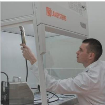
**HEPA FILTER INTEGRITY CHECKING**
