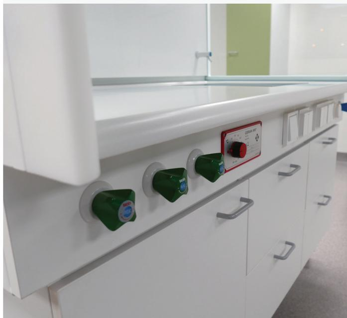
**The VISU fume cupboard with a low worktop (M-model) enables even large equipment and test arrangements. The fume cupboard can also be open to the floor.**
